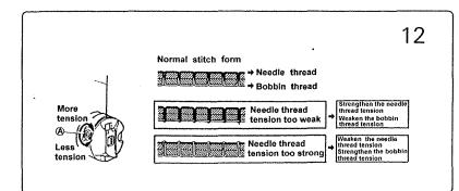
Thread tension should be determined in accordance with the stitches obtained by adjusting the tension of the bobbin thread and needle tension (Fig. 12).
