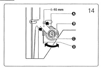
The tension of the needle thread: to be adjusted by turning the thumb nut.
